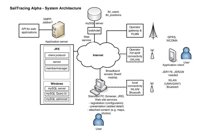
Figure 12 System architecture of the SailTracing application.
